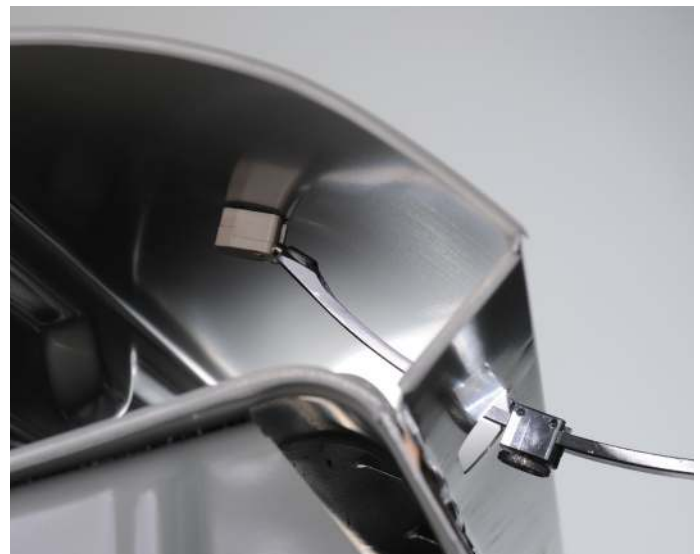
Car body in section to show how the probe V3FGA06H measures the EPD coating within the car body.
