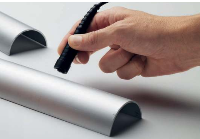
Measurement of anodized coating with the curvature-compensating probe FTD3.3.
