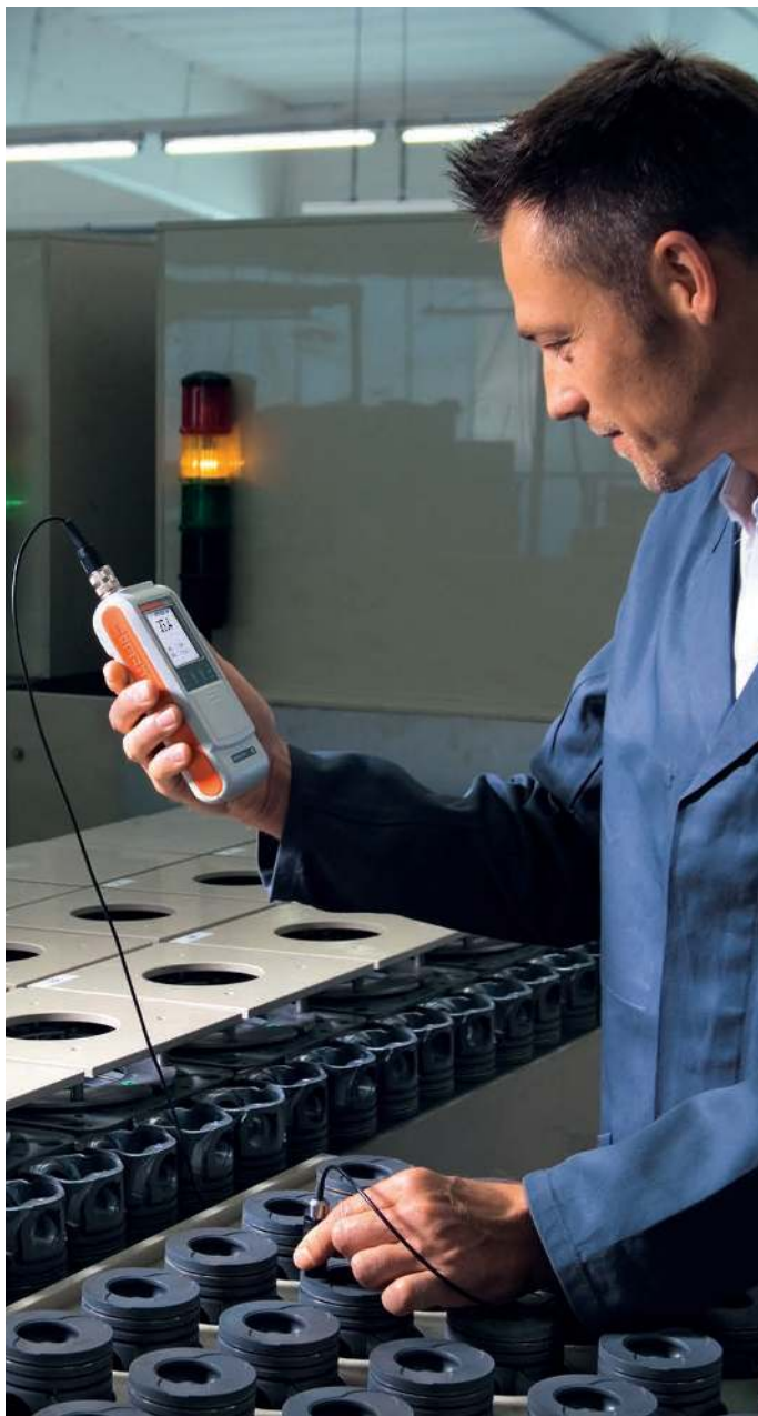
Quality monitoring on engine pistons after the manufacturing process using the FTA3.3H probe.
