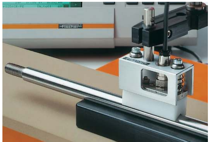
Automated measurement of the chrome coating on piston rods with the probe V2FGA06H.
